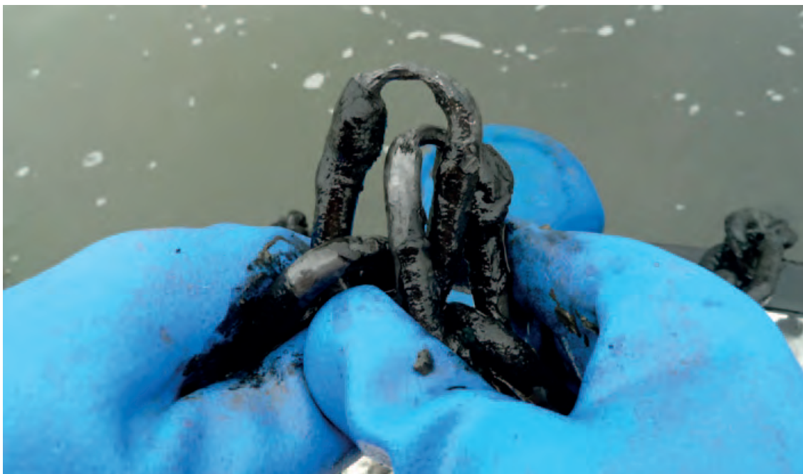
A routine inspection of a Licensed Mooring revealed that the Licence Holder had not been maintaining their mooring
